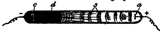
Fig. 43.—Discharge in a vacuum tube; a , anode; c , cathode; d , dark space round c ; s , flickering strip.
